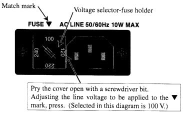
Fig. 1-3 Removing the Fuse Holder
