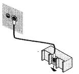
To the ground terminal (GND) on switchboards
