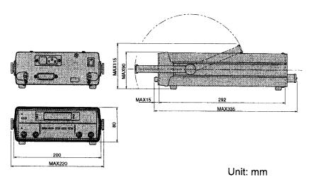
Fig. 7-1 KBM6010 External Dimension Diagram
