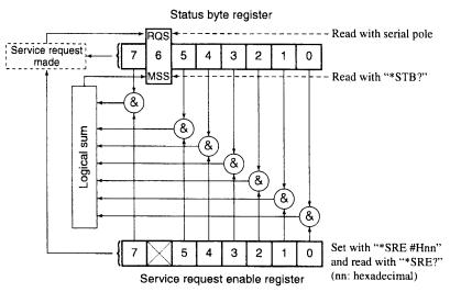
Fig. 4-3 Register Structure
