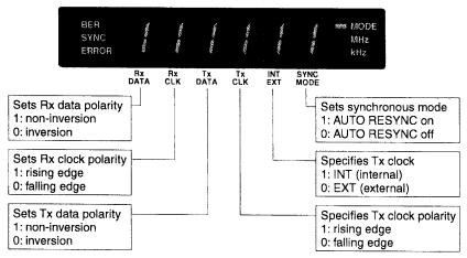
Fig. 2-10 Clock/Data/Synchronous Mode Setting Mode Display
