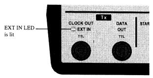
Fig. 2-1 TX CLOCK EXT IN LED
